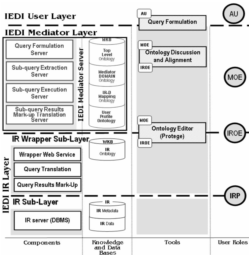
Figure 2. IEDI Clients and Servers along the layers of the architecture.
